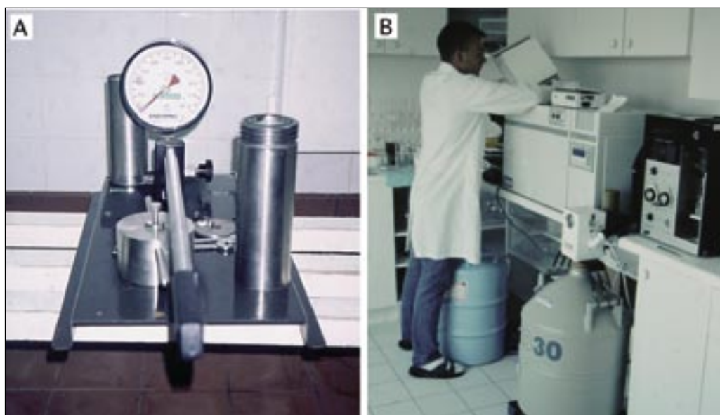
Figure 110: A – a device for exerting pressure on eggs to prevent chromosomal reduction through the suppression of meiosis. B – experiments in the cryopreservation of bivalve gametes and larvae.
