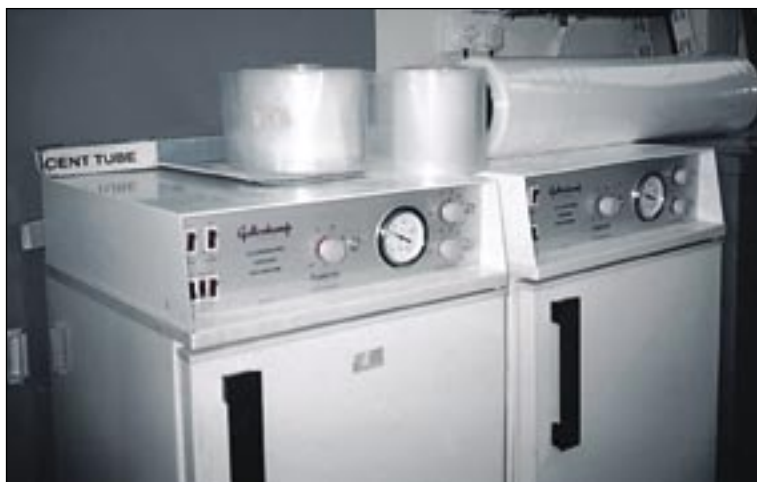
Figure 15: Illuminated, temperature controlled incubators for the maintenance of small algal cultures.
