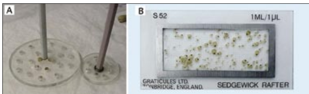
Figure 58: Equipment used in estimating numbers of larvae. A – perforated plungers for evenly suspending larvae in containers from which known volume sub-samples are taken in the estimation of larval numbers. B – a sedgewick rafter microscope slide, which has a chamber designed to take a 1 ml sample. The chamber has a grid marked on the base for easy tracking while viewing and counting larvae or spat in the sample. Similar slides can be made from transparent plastic.
