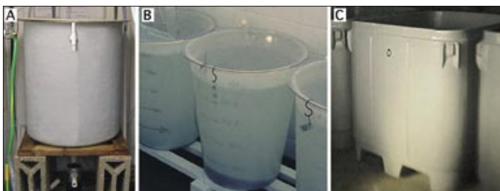
Figure 52: Suitable rearing vessels for embryo (and larval) development. A – 200 l steeply tapering conical fibreglass tank with bottom drain; B – 125 l polyethylene flat-bottomed tank; C – 1 000 l insulated polyethylene, square tank with rounded corners.
