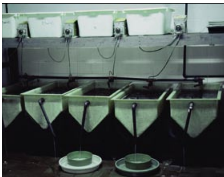
Figure 43: Experimental broodstock conditioning of Ostrea edulis . Note the green coloured sieves immersed in shallow trays to catch and retain larvae.
