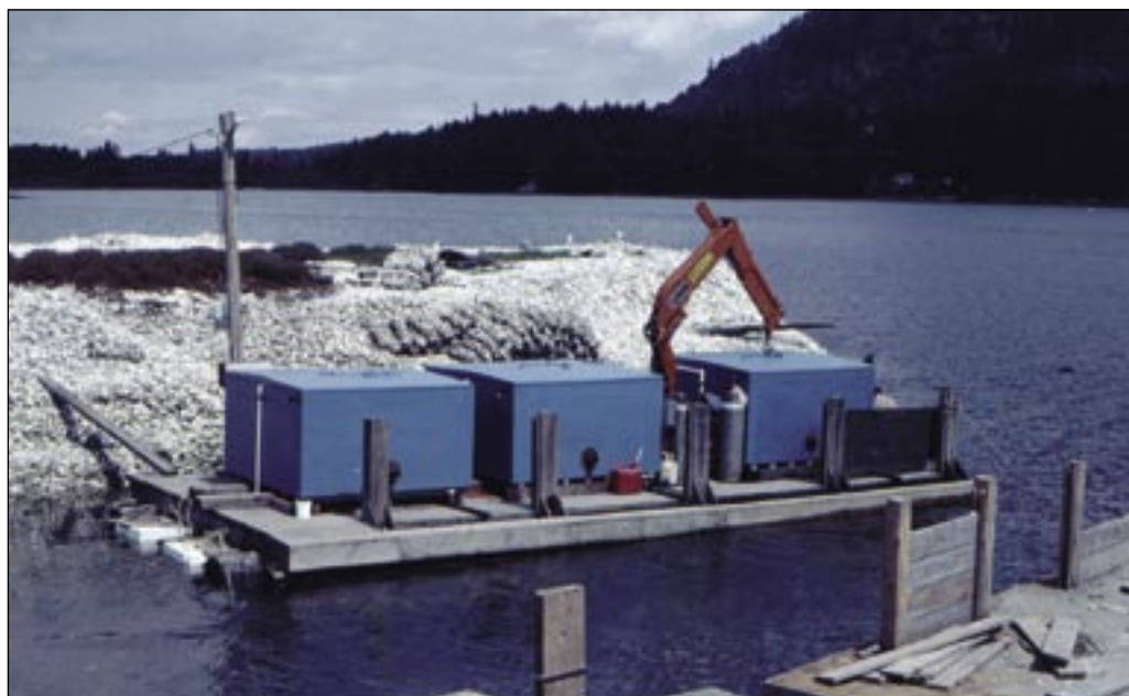
Figure 90: Setting tanks at a site in British Columbia, Canada. Note the loose cultch and vexar bags filled with cultch stacked on the bank behind the tanks. Refer also to Fig. 85, Part 5.4.3.2.
