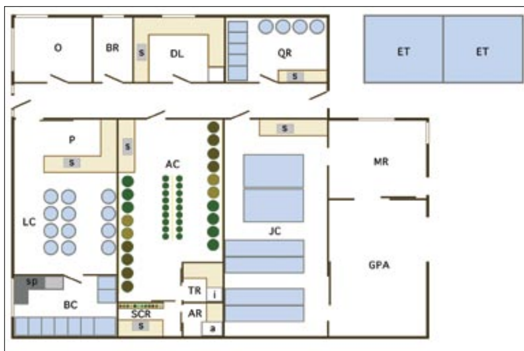
Figure 5: A generalized floor plan for a purpose-built bivalve hatchery (see the following text for explanation).
