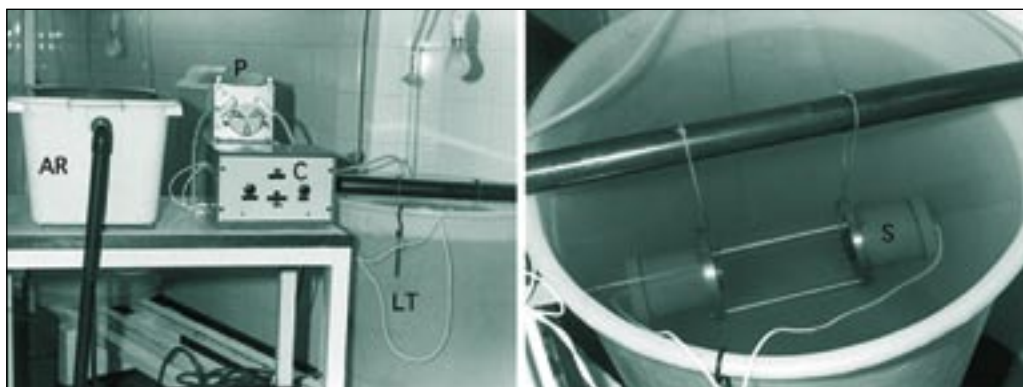
Figure 62: Experimental automatic control of food cell density in high-density cultures of bivalve larvae. AR – chilled, aerated algal reservoir containing the daily food ration; P – peristaltic pump which delivers the required amount of algae upon demand; C – control equipment containing a relay that switches the pump on when the sensor (S) detects a decrease in food cell concentration in the larvae tank (LT) below a certain pre-set threshold. This device utilizes an infra-red transmitter and receiver and could be greatly improved with modern electronics.
