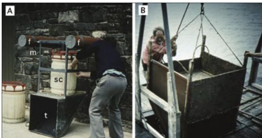
Figure 108: Tidal powered, floating upwelling systems – “FLUPSYS”: A – a small experimental unit showing the various components. The unit floats on the water surface buoyed by styrofoam filled flotation pipes (f). It swings about a single point mooring (m – one of two mooring brackets) to face the direction of the tide so that water is forced into the throat (t) of the device and up through the spat container (sc). The spat container has a mesh base and may contain a bed of spat or a stack of trays. The forced water flow is discharged at the rear of the spat container with provision to prevent the escape of spat. B – a commercial application of the principle where several large “FLUPSYS” are mounted in a raft.
